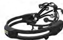
Fig. 4. Portable EEG system used to measure brain activity Photograph shows the EPOC headset manufactured by Emotiv Systems, Inc., San Francisco, U.S.A. Image source: http://www.emotiv.com/
